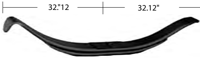
Trailer Two Leaf - High 6 3 / 4 " Arch 22,400 lb. GAWR Interchanges TRA2752 Part No. 324-00
