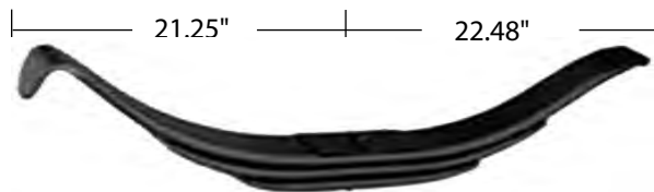
Trailer Spring, Three Leaf - High 5 1 / 2 " Arch Heavy Duty - 24,000 lb. GAWR Interchanges TRA-2740 Part No. 365-00
