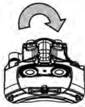
Type A Wheel Rotation (typically right hand)
