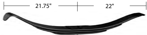
Trailer Spring, Three Leaf, Medium 3 3 / 4 " Arch Interchanges Reyco 21511-01 Part No. TRA3384
